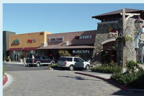
Pedestrian crossings should be delineated with a change in paving in shopping center parking lots.
