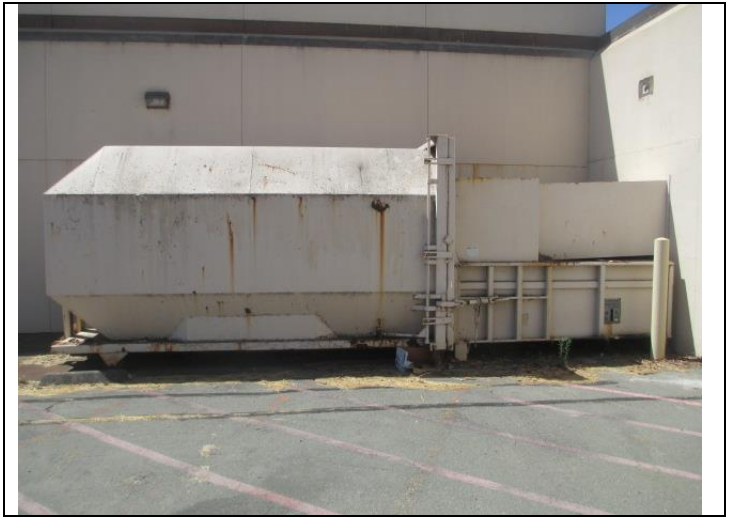
14. View of the hydraulic trash compactor.
