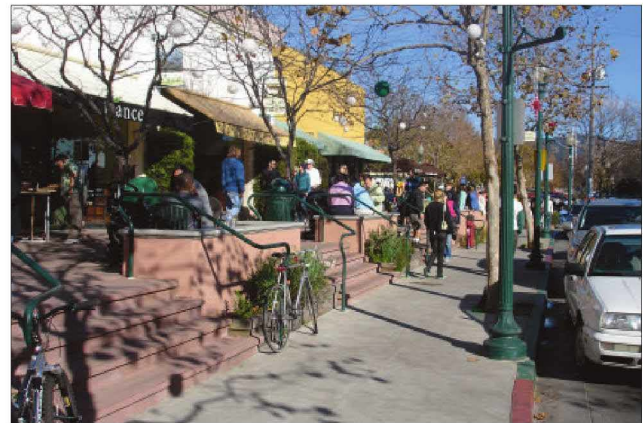
Terrace is used to accommodate a change in grade with low walls to provide seating.
