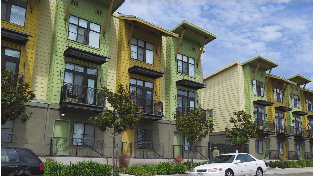
An Apartment Block articulated to appear as a series of townhouses with stoop entries.
